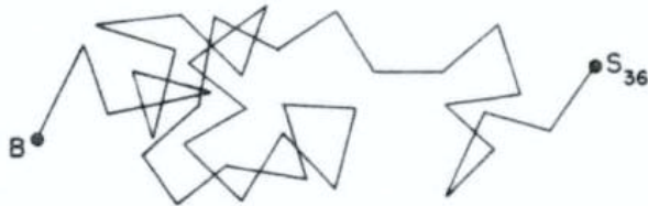
Fig. 41-6. A random walk of 36 steps of length l . How far is S_{36} from B ? Ans: about 6l on the average.
