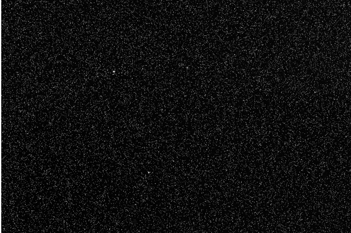
Figure 42: A typical ST-7E dark frame.
