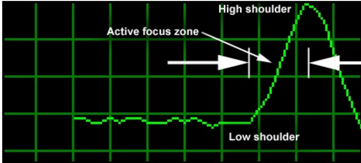
Figure 13: An ideal graph of the changes in Sharpness during an @Focus focusing run.
