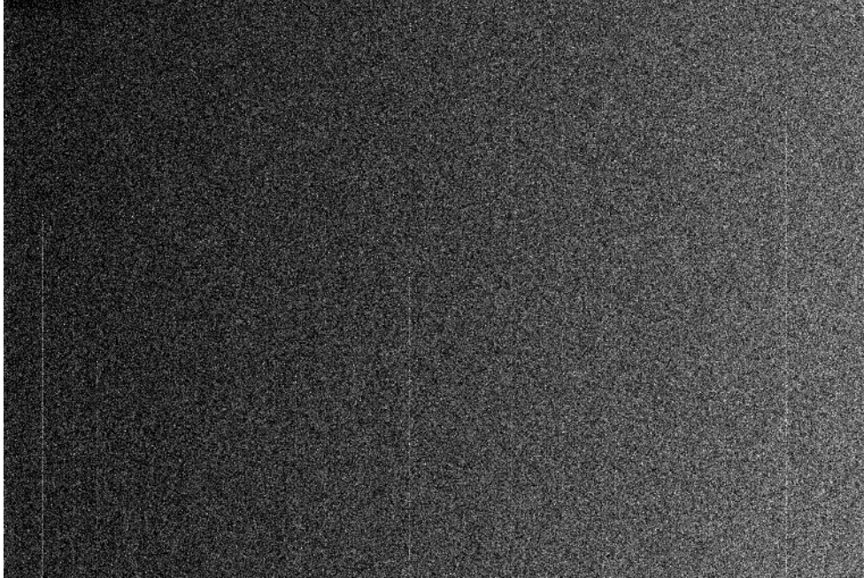
Figure 41: A bias frame from an ST-7E camera.
