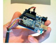
The wiring for a sketch involving the eyebrow switch is fiarly trivial. The 5v and ground pair go to +5v and GND pins. The three signal pins can be positioned anywhere that is specified by the sketch. For the purpose of several of my sketches, I used pins 2, 3 and 4.
